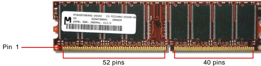
2. Insert the module straight down to the DIMM slot with both hands and press down firmly until the DIMM module is securely in place.
