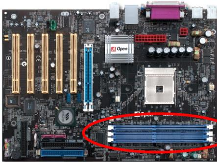
**Note:** According to the standard DDR400 specification from JEDEC (Joint Electron Device Engineering Council), it is regulated that DDR400 supports only 2x DIMM on the memory module for a maximum 2GB capacity, and DDR333 supports up to 3x DIMM for a maximum of 3GB capacity. Please be noted that K8T800 series motherboards follow this standard specification on memory as well.
