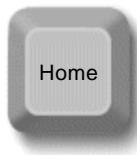
**Tip:** If your system hangs or fails to boot because of overclocking, simply use <Home> key to restore the default setting or you can wait the AOpen "Watch Dog ABS" reset the system after five seconds and system will auto-detect hardware again.
