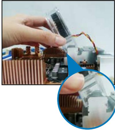
3. Carefully push down the fan until it snugly fits the heatsink, then connect the fan cable.
