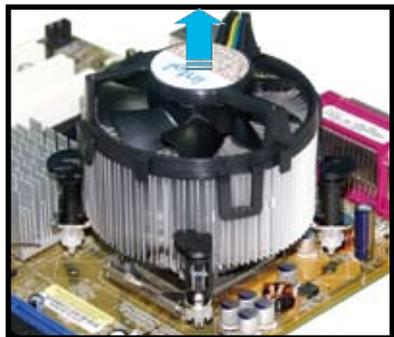
5. Rotate each fastener clockwise to ensure correct orientation when reinstalling.
