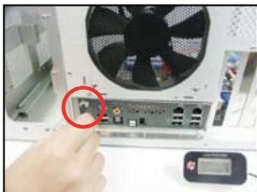
4. Plug the LCD Poster cable into the onboard connector labeled LCD\_CON.
