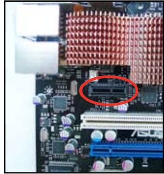
3. Align the card connector with the slot and press firmly until the card sits on the slot completely.
