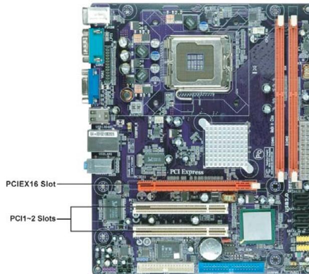
**PCIEX16 Slot** The PCI Express slot is used to install an external PCI Express graphics card that is fully compliant to the PCI Express Base Specification revision 1.0a.
