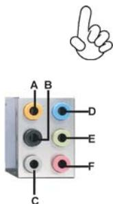
This motherboard may adopt 8-channel audio ports that correspond to the A, B, C, and E port respectively. In addition, all of the 3 ports, B, C, and E provide users with both right & left channels individually. Users please refer to the following note for specific port function definition.
