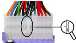
With ATX v2.x power supply, users please note that when installing 24-pin power cable, the latches of power cable and the ATX1 match perfectly.
